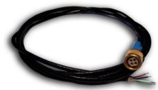
2266: The case's integrated connector shells, pins and sockets are gold plated brass. The 4PIN-CAB cable consists of four 30 AWG (7x38) silver-plated copper wires with PTFE insulation surrounded by a braided shield. The black FEP shield jacket has a nominal outer diameter of 0.100".
